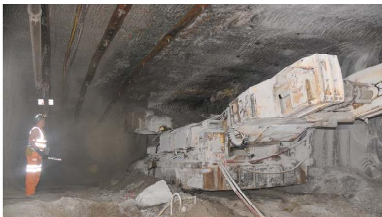
**Figure 2:** Mining machinery accessing the polyhalite seam.
