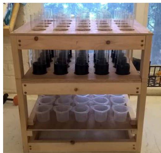
Figure 2: Apparatus for the determination of the relative rates of dissolution of different sulphur-containing fertilisers.
